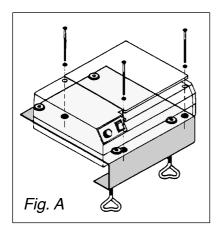
To mount either the #60514 MicroLux Multi-Saw or the #50304 MicroLux 2" Table Saw, use the 3 long screws and washers provided to attach the plate to the bottom of the saw housing, as shown in Figure A.
