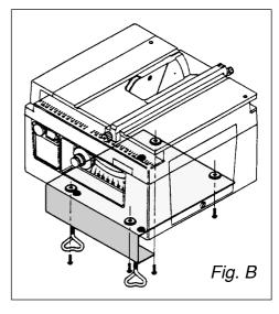
To mount the #80463 Tilt Arbor Table Saw, use the four short screws provided to attach the plate to the bottom of the saw housing, as shown in Figure B.
