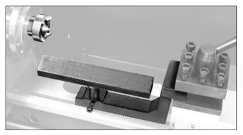
Install Tool Rest in Tool Post as shown. Tighten Cap Screws securely.
