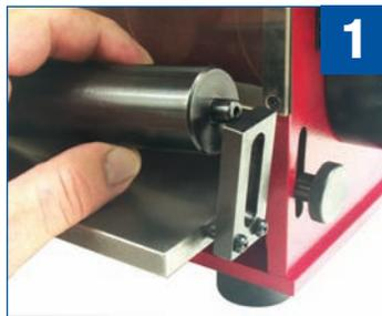
Then, tighten the screws and make sure the roller “floats” vertically freely. The purpose of the roller is to hold the wood sheet in contact with the table (this is the in-feed side of the machine).
