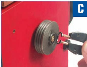
Remove the pulley by sliding it off the shaft.
