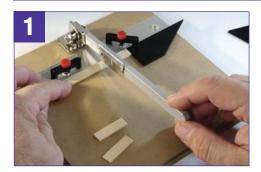
Use Chop It as shown above to cut a set of stripwood pieces to the same length. Use the right-angle gauge as a stop bar.
