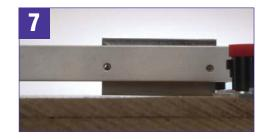
For better cutting action, the blade is deliberately set at a slight angle to the base board to provide a slight slicing action. Be sure to press down far enough to completely cut through the workpiece.
