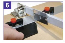
If so desired, use the chopper to cut off a small tip of the angle gauge to allow closer positioning of the gauge to the cut line.
