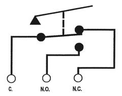
C = Common N.O. = Normally Open to Common N.C. = Normally Closed to Common
