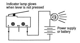
Note: Do not overheat the switch terminals while soldering wires to them; otherwise, the switch will be damaged.
