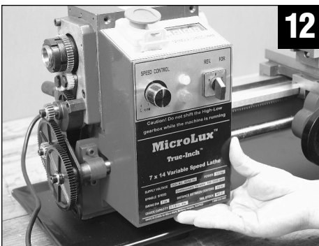
Install control box to headstock with 4 screws. Be sure grommet is properly engaged and wires cannot foul the lead screw.
