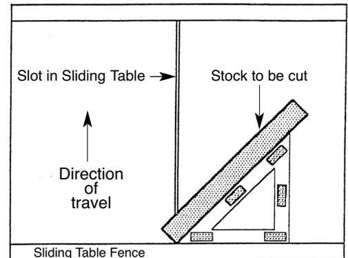
When cutting angles, position stock against triangles as shown above.
