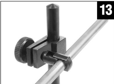
**13** Install the brass nozzle tube through the clamp and reinstall on the support rod. Tighten the knob until the clamp just grabs the support rod (over-tightening will damage the brass tube).
