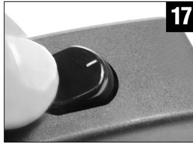
**17** Make sure the switch on the power cord is set to OFF (press the end of the button opposite the "I").
