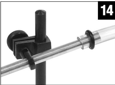
**14** Install the free end of the clear tubing (with the O-ring) over the plain end of the brass nozzle tube. Move the O-ring to the location shown to hold the clear tubing on the brass nozzle tube.
