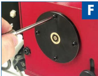
Remove the bearing plate and drum (you may have to tap on the opposite end of the shaft with a wood block to release it).
