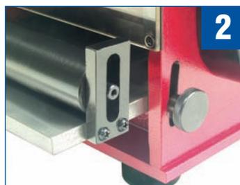
The thumb screws located on each side of the machine lock the table in position.
