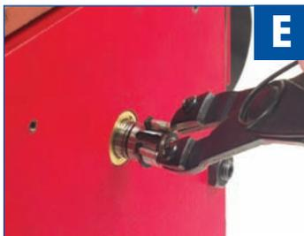
On the opposite side of the machine, remove the 4 screws holding the bearing plate to the red machine frame.
