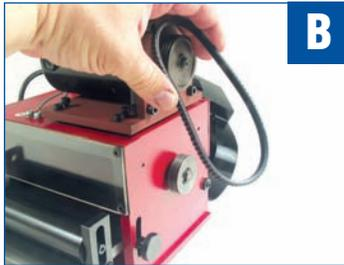
Remove the outer C-clip from the pulley shaft.
