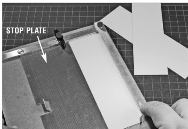
Position the stop plate the desired distance from the inside edge of the clamp bar. To assure squareness, be sure the stop plate is in good contact with one fence or the other, then clamp the stop plate in place (you can
