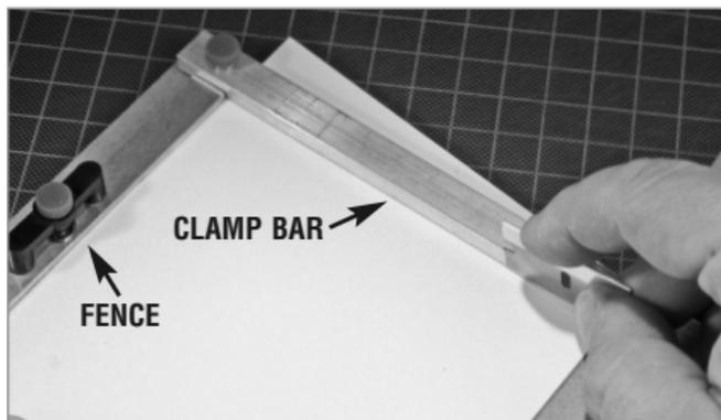
To square-up a workpiece, remove the stop plate, then loosen the two knobs that hold down the clamp bar. Now slide the workpiece underneath the clamp bar. Position the
