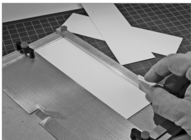
Duplicate parts are made by leaving the stop plate in position when you load and unload more workpieces.
