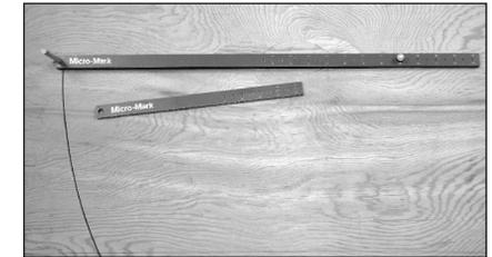
Short bar is marked for radii from 7" to 11" in half-inch increments. Long bar is marked for radii from 11-1/2" through 23" also in half-inch increments. Press fit pencil into large hole at end of bar. Insert ball-end pin through hole corresponding to your desired radius. Press pointed end of pin into layout baseboard at desired center of track curvature. Swing the bar and use the pencil to draw the arc on the track roadbed.
