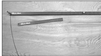
Short bar is marked for radii from 7" to 11" in half-inch increments. Long bar is marked for radii from 11-1/2" through 23" also in half-inch increments. Press fit pencil into large hole at end of bar. Insert ball-end pin through hole corresponding to your desired radius. Press pointed end of pin into layout baseboard at desired center of track curvature. Swing the bar and use the pencil to draw the arc on the track roadbed.
