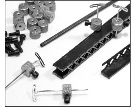
Pin collars are special fittings that lock into position on straight or T Pins. They hold parts in place during assembly when there is no room for traditional spring, bar or screw-type clamps. Pin collars work great when parts are fragile, since they hold with very little pressure.
