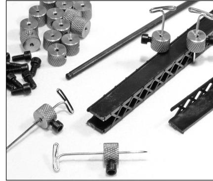
Pin collars are special fittings that lock into position on straight or T Pins. They hold parts in place during assembly when there is no room for traditional spring, bar or screw-type clamps. Pin collars work great when parts are fragile, since they hold with very little pressure.
