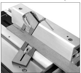
Attach the high fence to the standard fence using the three round head machine screws as set screws. The large side of the high fence should face the blade. Make sure the fence is seated fully in contact with the saw table. Tighten the screws gently (just enough to hold the fence); excessive torque will cause the high fence to shift from a vertical position and permanent damage may occur.
