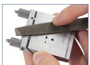
Use the stop bar as shown in the picture below to make workpieces of duplicate length.
