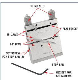
Loosen the thumb nuts to open the jaws. Insert your workpiece into a suitable groove to hold it at the needed angle. Then, gently tighten the thumb nuts until the workpiece is securely held without being crushed. Note: Flat stock should be placed against the flat fence to hold it "square" to the jaws.
