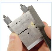
Lay your saw blade up against the surface of the jaws to guide the cut. After the cut is made, run your file across the surface to smooth out the cut and finish to size.
