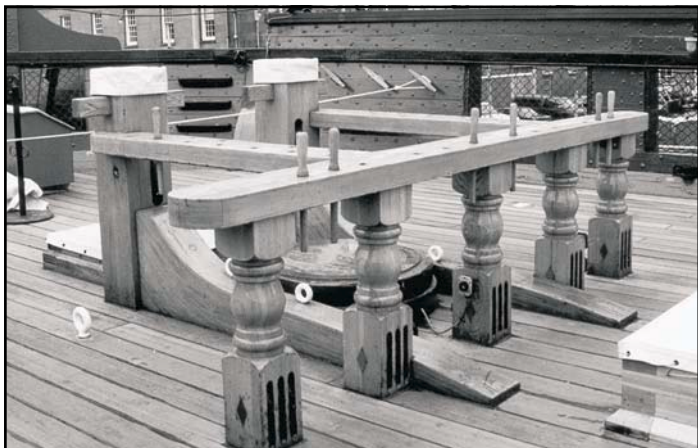
FOREMAST FIVE RAIL undergoes restoration. Note the triple sheaves in the base of each stanchion. Three levels in the bulwark are normally used for belaying large lines.
