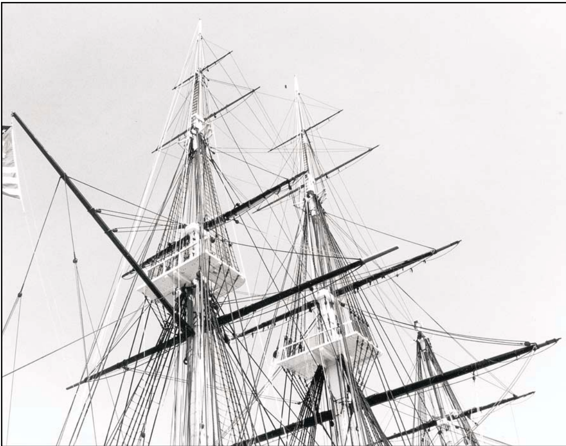
MIZZEN AND MAIN TOPMAST, TOPGALLANT, AND ROYAL MASTS. A hurricane in 1998 broke the foremast's topgallant and royal masts. View looks from the stern forward. Spanker was bent to the gaff on the mizzenmast. Sailors went quickly aloft using the ratlines on the shrouds and topmast shrouds.
