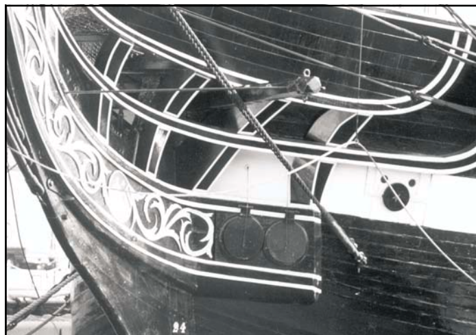
HEAD RAILS. Notice covers over hawse pipes.
