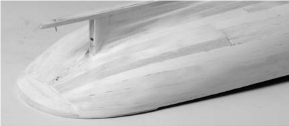
Photo 8: The completed fantail stern. Sanding and filling has begun
