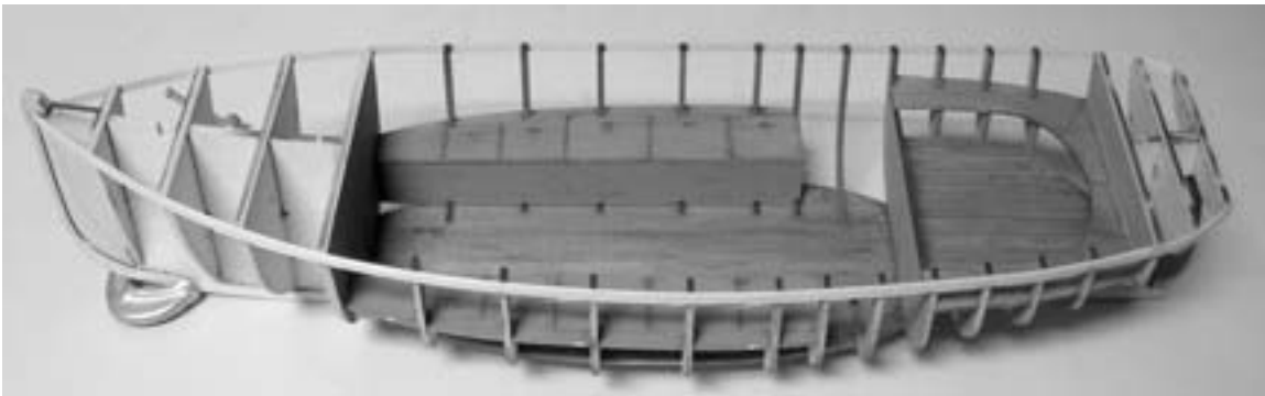
Photo 2: the completed hull structure ready for planking
