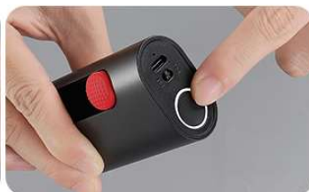
5. After use, click the round button at the bottom to shut down
